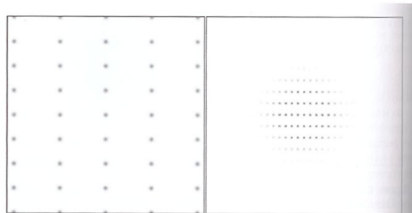
Figure 2.9 ▶ Lattice of spheres (left) and its diffraction pattern (right). If you look at the pattern and blur your eyes, you will see the diffraction pattern of a sphere. The pattern is that of the average sphere in the real lattice, but it is sampled at the reciprocal lattice points.
